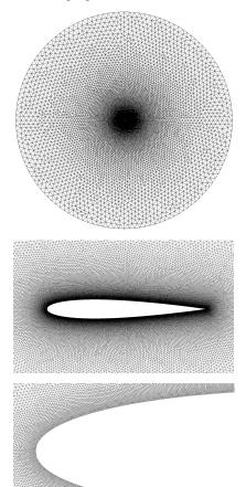
Cell size is the finest near the airfoil and grows proportional to distance from the airfoil surface. Cell size is controlled with combination of Field in NACA0012\_O.geo as shown below.:
